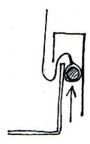
As the stainless band is pushed into place the canvas is pulled taut and seen from the outside the stitch line should be more or less flat with the caravan roof. You can use the G-clamps and wooden blocks on the corners of the steel band to help pull it into place.
